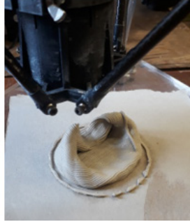
Figure 5. Ceramic Object collapse caused by unsuitable nozzle size and printing speed
