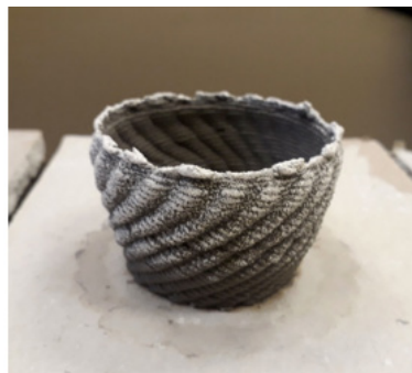
Figure 30. Printed Egyptian faience drying, efflorescence process
