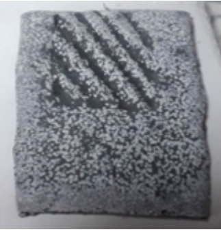
Figure 13. Sodium salts start to form Figure 14. Efflorescence process
