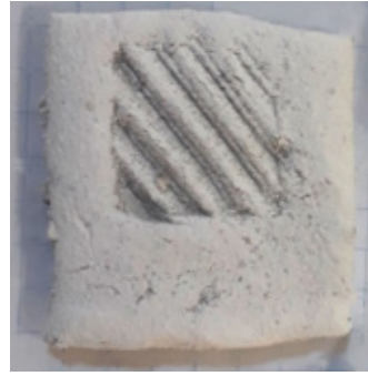
Figure 13. Sodium salts start to form Figure 14. Efflorescence process
