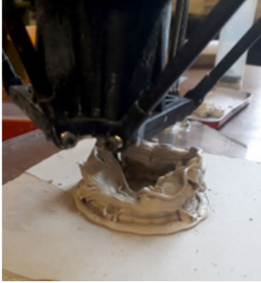
Figure 4. Stoneware clay wasn't prepared good enough. Air bubbles in clay caused clay object to collapse
