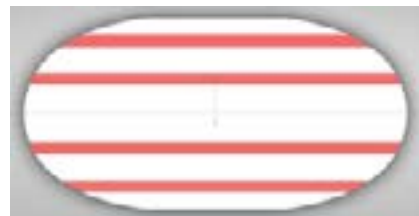
Figure 3. Representation of footprint area (white zone, in contact) of aircraft tire with rib tread (red zone, non-contact).
